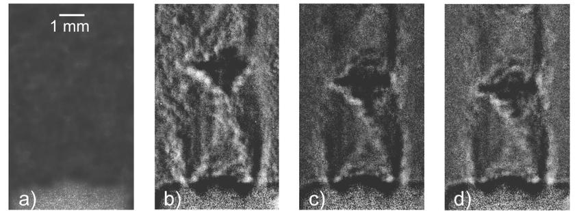
Figure 3 - a) background, b) supersonic jet M = 2.78 , c) supersonic jet M = 1.89, d) supersonic jet M = 1.79
