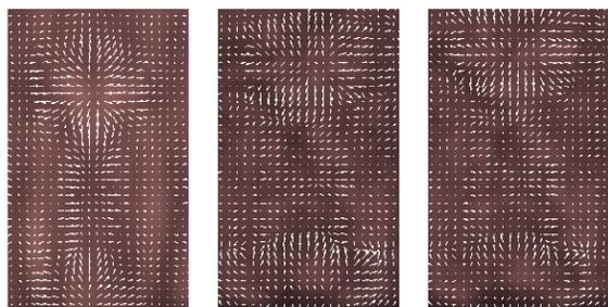
Figure 4- Displacement field of the jet at three different Mach numbers obtained through the cross-correlation between the images shown in Figure 3, a) with b), a) with c) and a) with d).
