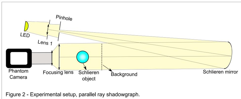
Figure 2 - Experimental setup, parallel ray shadowgraph.
