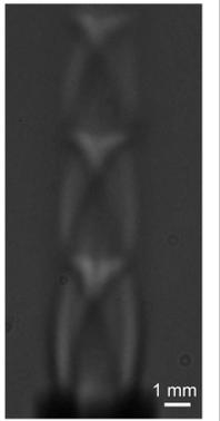
Figure 1.- Shadowgraph of the supersonic jet.
